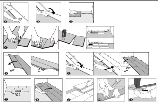
1. First row, first plank: After thoroughly cleaning the subfloor, you should begin laying from left to right. Position the first plank so that grooved edge is facing you. Place the floorboard 1/4" / 6 mm from the left wall. Use spacers between the wall and the floorboard.
