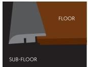
**REDUCER** is used when ending the flooring onto a surface such as concrete.
