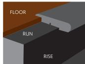
**STAIR NOSE** is used when ending flooring at the top of either a landing or downward staircase.
