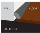
**QUARTER ROUND** is most commonly applied to cover the expansion gap between the flooring and the wall.
