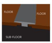
**T-MOLD** is used when joining two floors of equal height, such as in a doorway, between two rooms or in a large area where the maximum length/width is exceeded.
