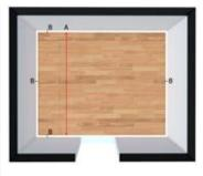
Note that the dimensions of the skirting board must never determine the size of movement joints. With large floor areas, the skirting board must therefore be selected on the basis of the required size for the expansion joint and not vice versa.
