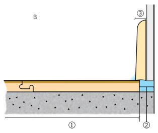
Movement joint x 1.5 = skirting board minimum thickness in mm
